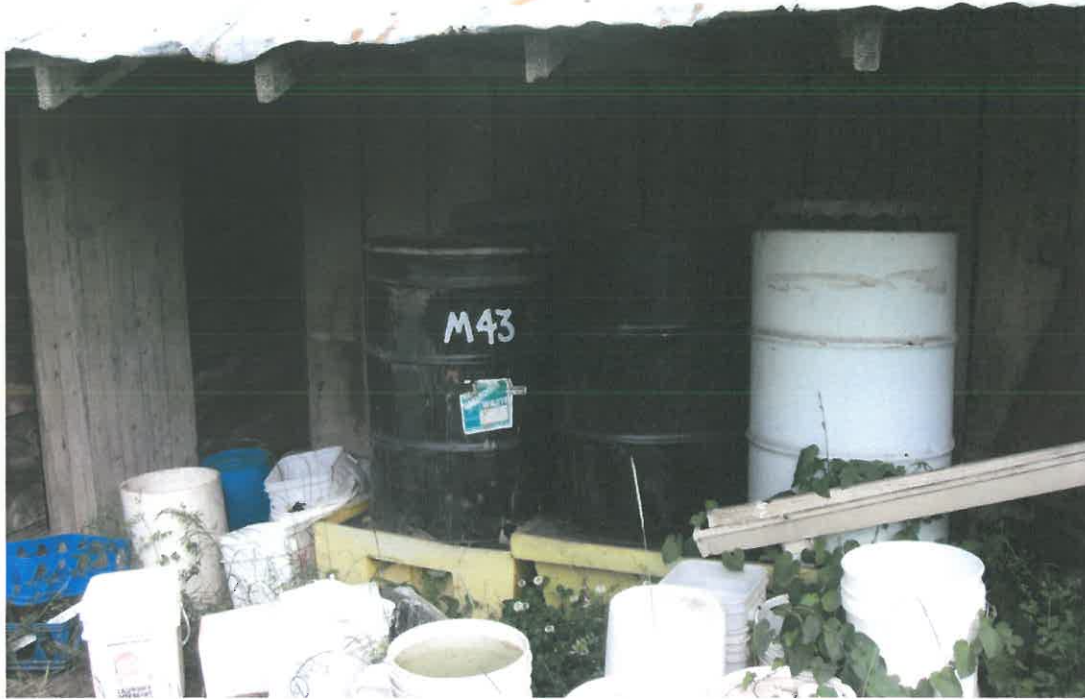
Photograph 7: Waste oil drums on secondary containment pans located under shed on southwest quadrant of subject property.
